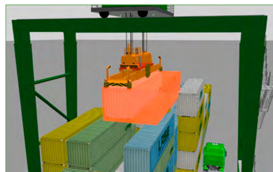
LaseLCPS-3D solution: virtual cube detects potential collision
