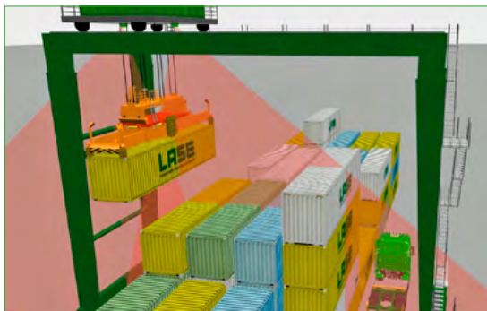
LaseLCPS-2D solution: 2-dimensional scan during trolley drive
